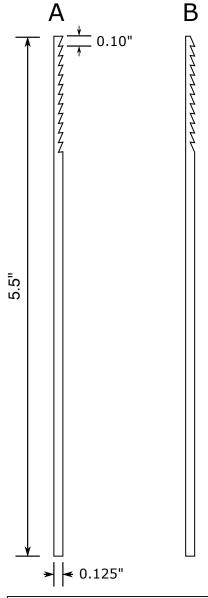
Handle is wood, with two 3/16" holes drilled through the tang of the float to accept 3/16" brass pins. The teeth are filed in with a triangular file at perpendicular or slight negative rake. Tooth depth is  $\sim 0.1$ ". (A) shows pattern for pull-stroke float, (B) for push-stroke float.
