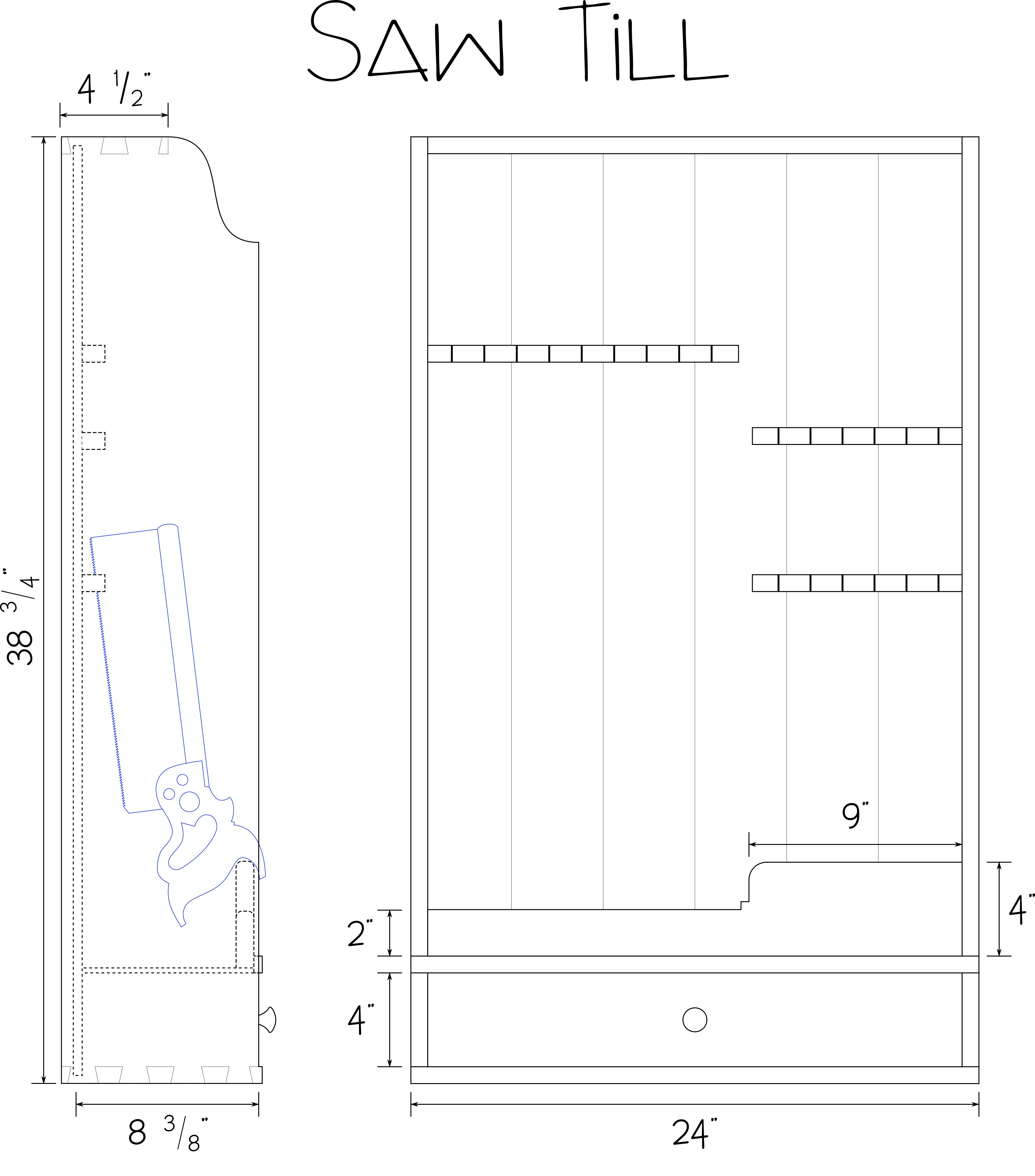
CARCASS is  $^{3}/_{4}$ " pine, as is front rail and drawer front. Back is paneled from shiplapped and beaded pine  $^{3}/_{8}$ " thick. Till is hung from a  $^{1}/_{2}$ " french cleat.
